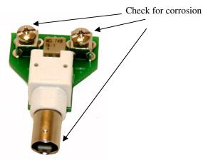
Check antenna loop for proper resistance. Disconnect the antenna loop from the balun terminals and measure between the two ends of the loop. It should read about 470 ohms. If it is within +/- 50 ohms then the reading is ok. If you see large resistance or an open it means there is a break in the loop.
